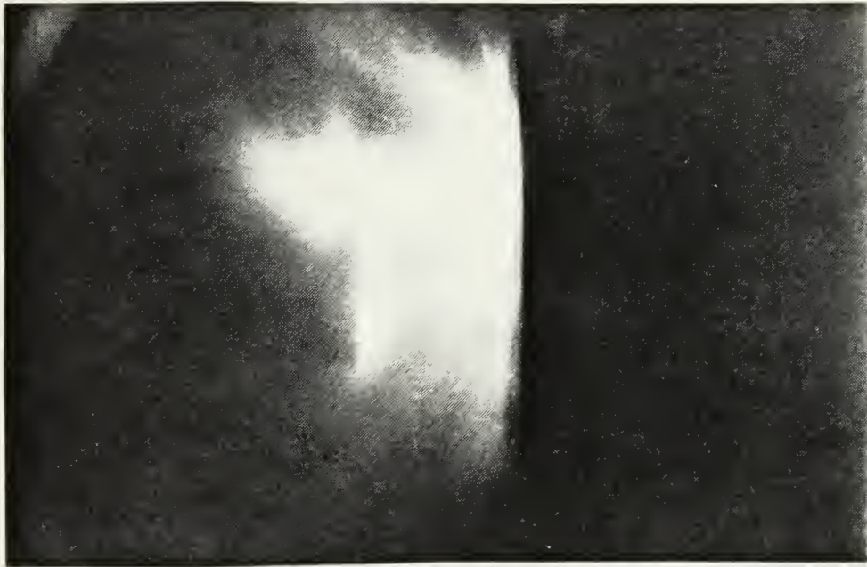
Figure 5.2 Time lapsed photograph of a 75 kV shot using a 10% transmittance neutral density filter. Notice intense spots on cathode surface (cathode spots).
